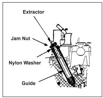
5. While holding hex end of extractor with wrench, turn jam nut with another wrench to remove ground electrode shield.
