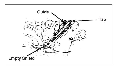
4. Once the ground electrode is tapped, insert the extractor through the guide and thread into the ground electrode shield. Place nylon washer and jam nut onto threaded shaft.
